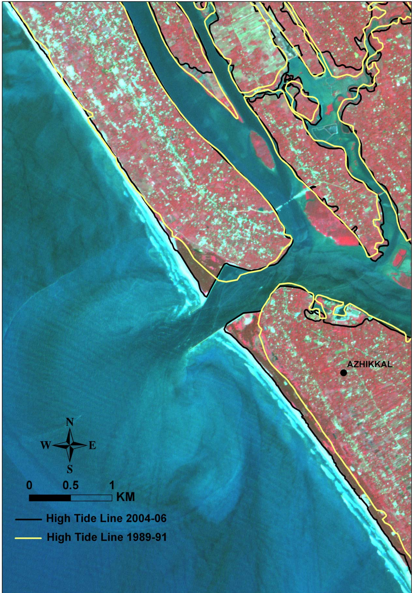
Plate 5: 2011-12 LISS IV image overlaid with high tide line of 2004-06 and 1989-91, showing the changes at Valapattanam River mouth near Azhikkal in Kannur District due to the construction of break waters (49M05NW).
