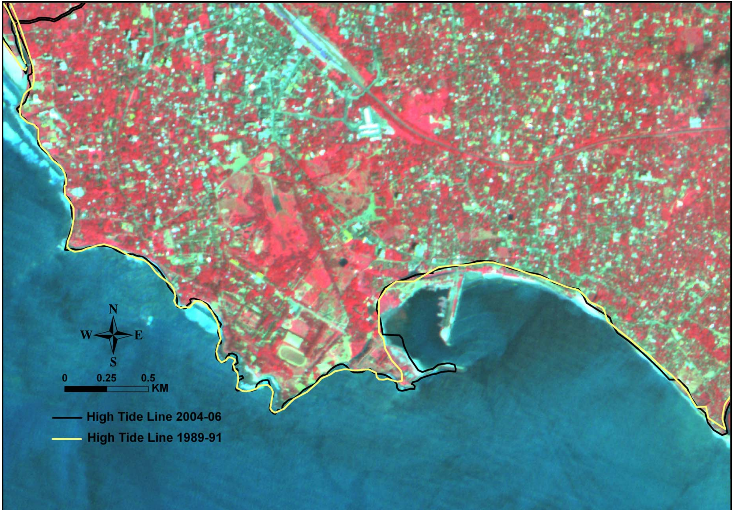
Plate 6: 2011-12 LISS IV image overlaid with high tide line of 2004-06 and 1989-91, showing the coastal changes at Kannur due to the construction of break waters (49M05SW and 49M05SE).
