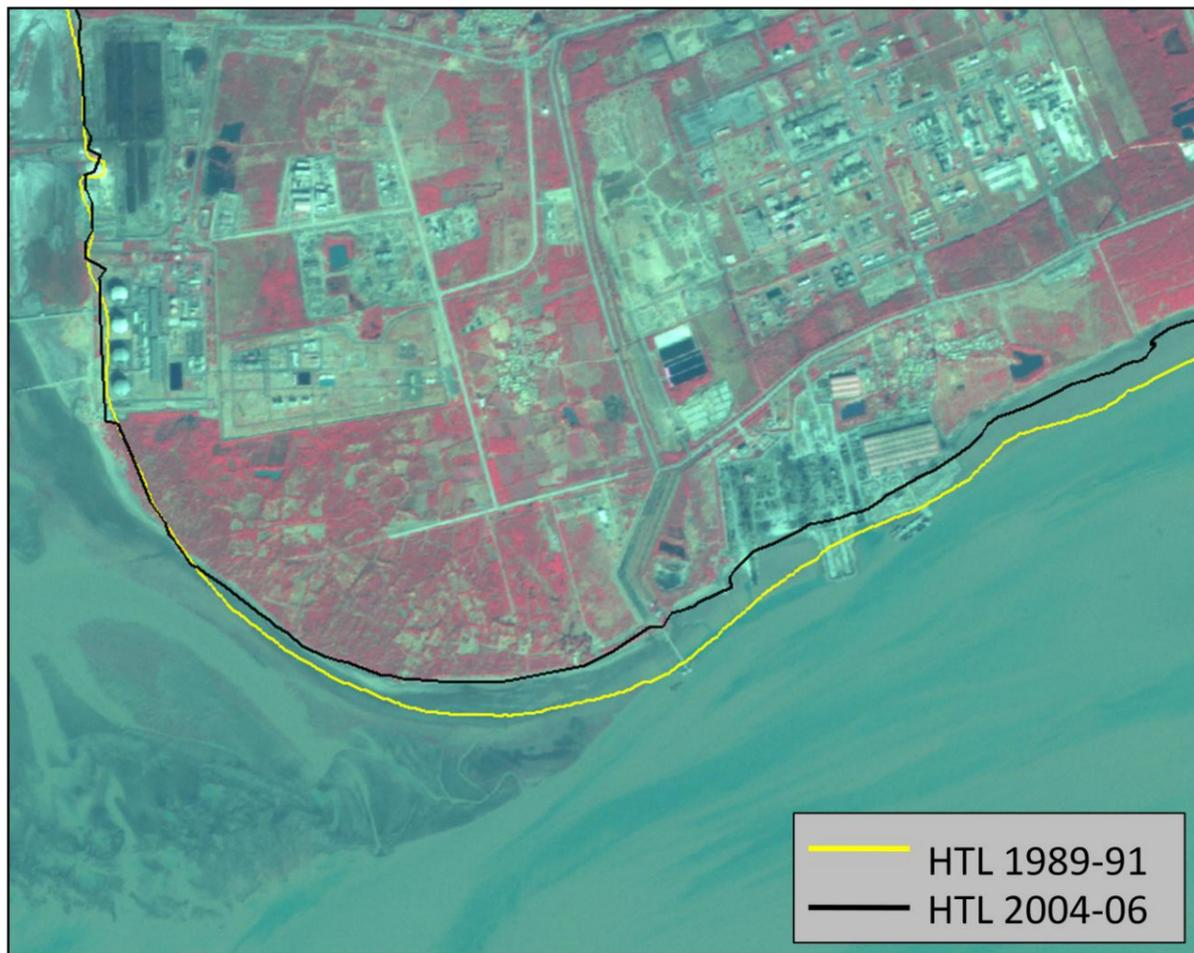
Plate No. 7: Coastal stretch along south of Dahej, Bharuch district (Map Sheet no. 46C10NW) showing eroding areas (Image: 2011 LISS IV).
