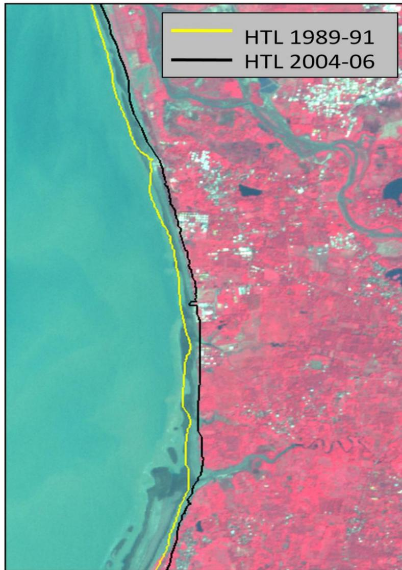
Plate No. 11: Coastal stretch along Kosamba & Tithal, Valsad district (Map Sheet no. 46D14SE) showing eroding areas (Image: 2011 LISS-IV).
