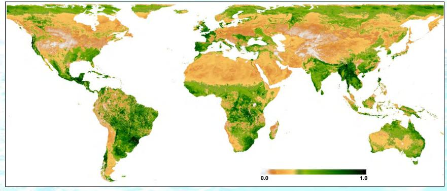
Above image shows first Global Normalized Difference Vegetation Index (NDVI) composite of five-day (20-24 Jan 2023) duration from EOS-06/OCM-3 sensor. These global NDVI datasets will be useful as input to different global vegetation, biogeochemistry and hydrological modelling. The datasets will also be useful in characterizing land surface biophysical properties and processes.
