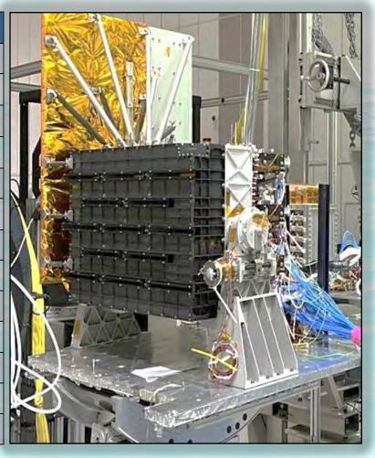
Five new bands have been included in EOS-6/OCM-3 as an advancement over OCM-1 and OCM-2 (satellites of ISRO). There are 3 new bands for fluorescence, 1 new band for specific type of nitrogen fixing bloom detection and 1 new band for turbid water atmospheric correction for better understanding of oceans.
