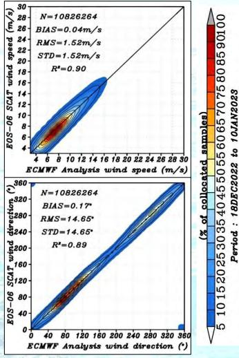
Validation of SCAT-3 Leve-2B wind products with NWP analysis from European Centre for Medium Range Weather Forecast (ECMWF) Validation of SCAT-3 is carried out using following technique:
