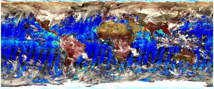
OCM-3 has unique characteristics of observing global ocean and land surface due to its high temporal resolution due to large swath with a moderate spatial resolution. Above image shows four-day composite image of land overlaid with three-day ocean chlorophyll showing a unique advantage of OCM-3 as a global sensor.
