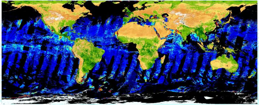
OCM-3 has unique characteristics of observing photosynthetic activity over global ocean and land surface due to presence of visible – near infrared spectral bands. Above image shows four-day composite NDVI image of land overlaid with three-day ocean chlorophyll composite showing a unique advantage of OCM-3 as a global sensor.
