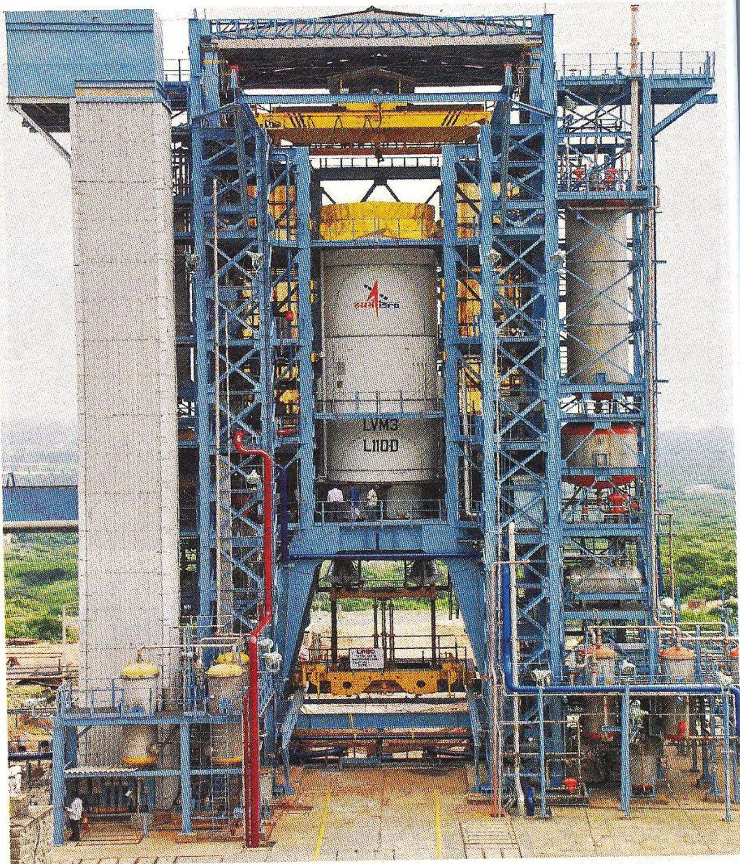
The L-110 stage of GSLV Mk-III undergoing final preparations for testing at the test stand at Mahendragiri, near Nagercoil, in Tamil Nadu. It is called L-110 stage because it is powered by 110 tonnes of liquid propellants. — PHOTO: ISRO
