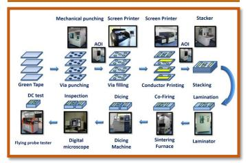
Space Applications Centre (SAC) of Indian Space Research Organisation (ISRO) has developed Low Temperature Co-fired Ceramics (LTCC) Multi Chip Module (MCM) and package fabrication technology. SAC's LTCC foundry process is qualified for space use. Its Design Rule Check (DRC) and Process Design Kit (PDK) features are unique for any LTCC foundry, globally.
