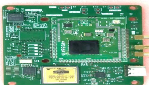
Credit Card size Receiver Module (57mm x 68mm)
