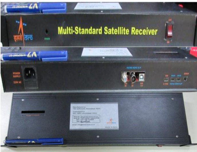
Integrated module, size:1U (can be further decreased by vertical PCBs stacking)
