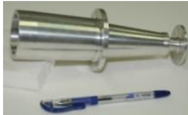
Profile corrugated horn at Ka band
