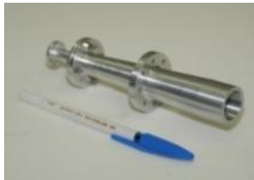
Profile corrugated horn at V band
