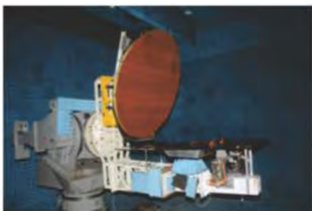
2.4m x 2.2m C-Band Tx-Tx DGR Antenna with Spacecraft mock-up and MLI Blanket
