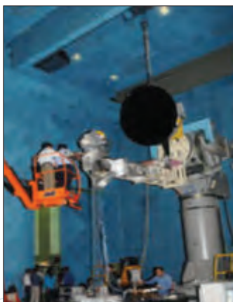
Antenna closed loop tracking test
