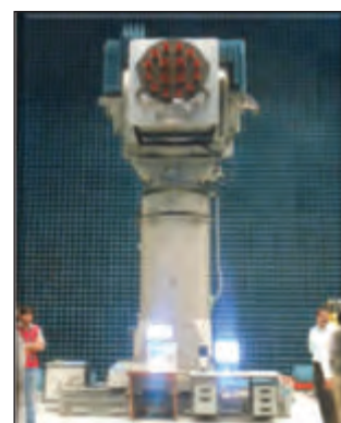
IRNSS 1E: Delay Measurement of Helix Array Antenna
