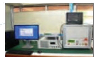
Automated Test Set up for Bulk Cable Injection tests CS114, 115 & 116 as per MIL-STD-461E
