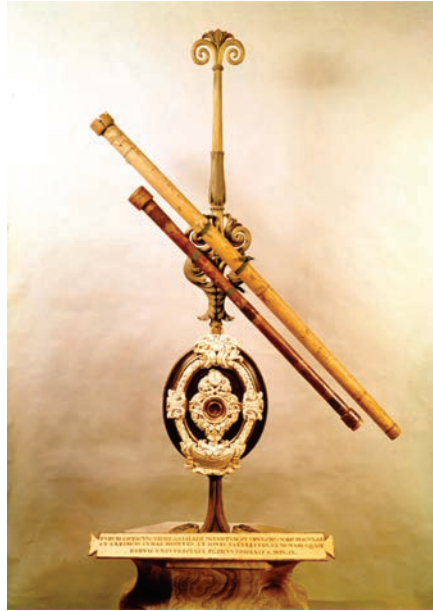
Fig.2.5: Galileo's 20x telescope
